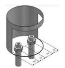
Plenum nozzle (P/N 93482 Orange Ring) can protect plenums up to (**10'**) long and (**48''**) wide, with either a single inclined
