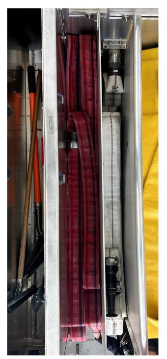
Now build a 100ft hose bundle, just like we do on our pre-connects, and leave a tail, as shown. Connect that to the male end sticking out the back of the truck.
