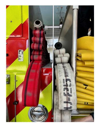
First, place 100 feet of hose flat loaded with a loop at the bottom:
